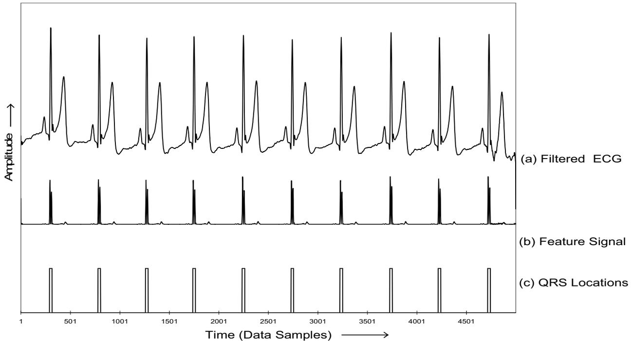
Figure 4. QRS detection for record MOI\_099
