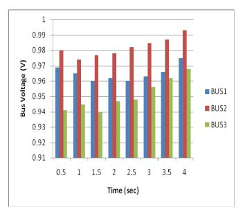
Figure 4: Bus voltages with STATCOM
