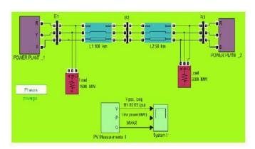
Figure 1.Simulink model without STATCOM
