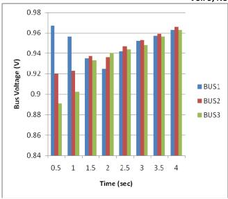
Figure 3: Bus voltages without STATCOM
